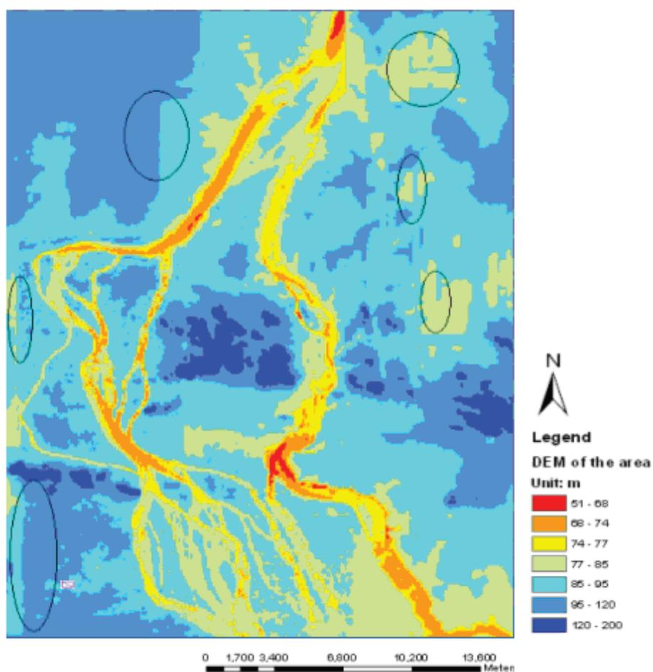
Figure 6. The newly developed DEM of the Siphandone wetlands, Lao PDR
