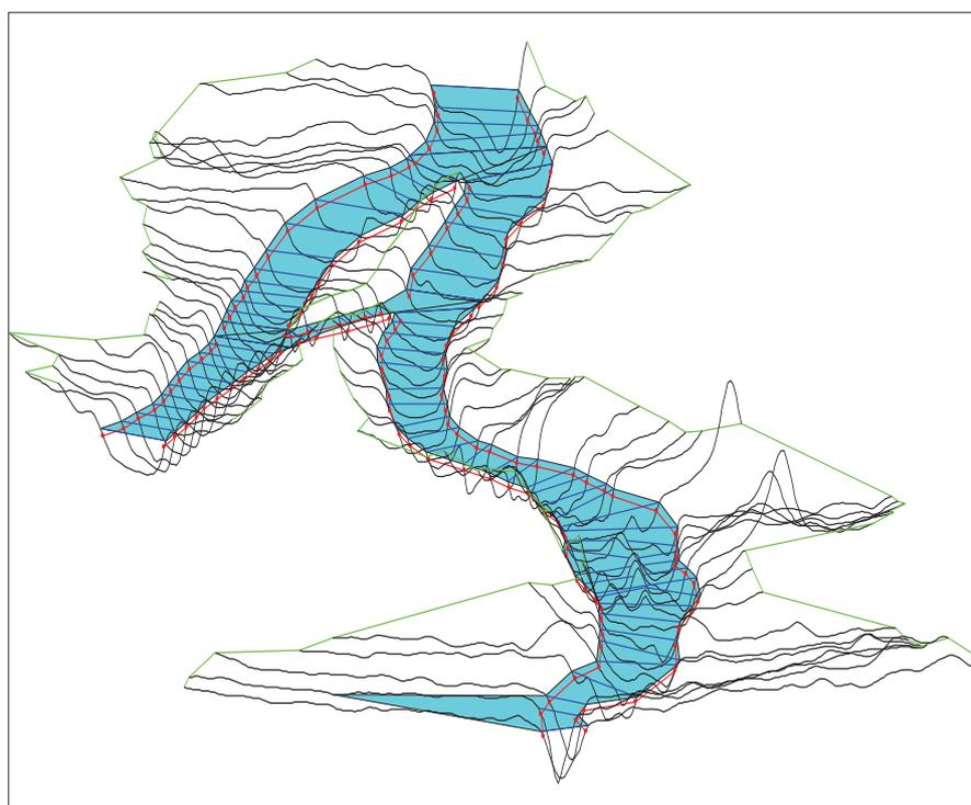
Figure 10. Flooding pattern according to three scenarios of the land cover pattern. Blue colour is the modelled channelized flow, the green lines indicate expected floodplain and red lines indicate the channel banks
