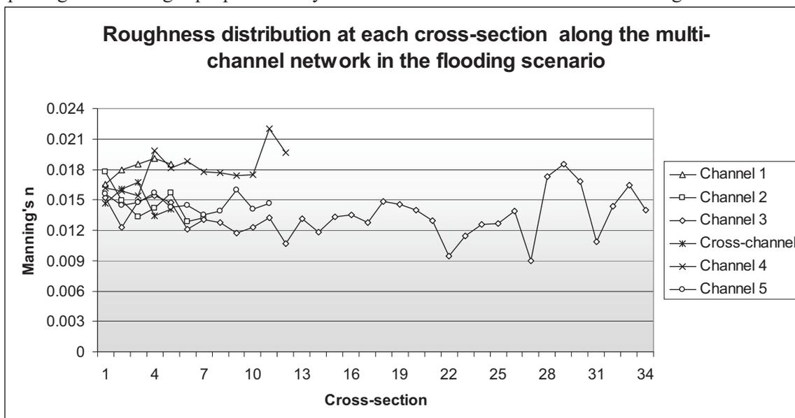
Figure 9. Hydraulic roughness distribution along the multi-channel network in the flooding scenario
