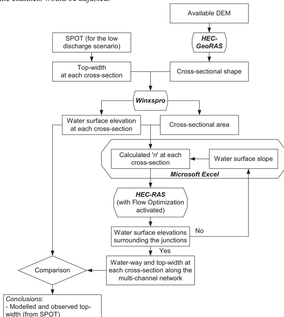
Figure 3. Routine to calibrate the HEC-RAS model for the low discharge scenario
