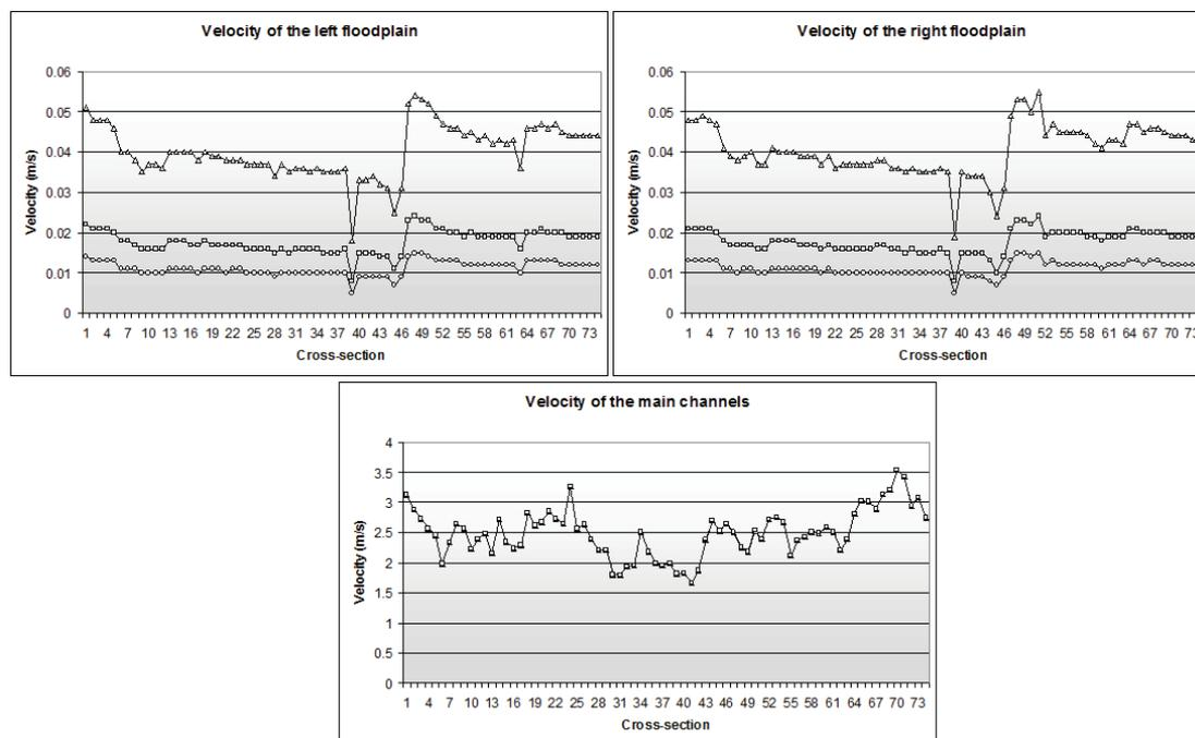
Figure 11. Velocity of the left-floodplain, channel and right-floodplain in different scenarios of the land cover pattern along the multi-channel network; square-symbol represents the present-day hydraulic roughness of the floodplain while triangle- and round-symbol represent the hypothetical cases where all areas were covered by rice paddy and dry forest, respectively
