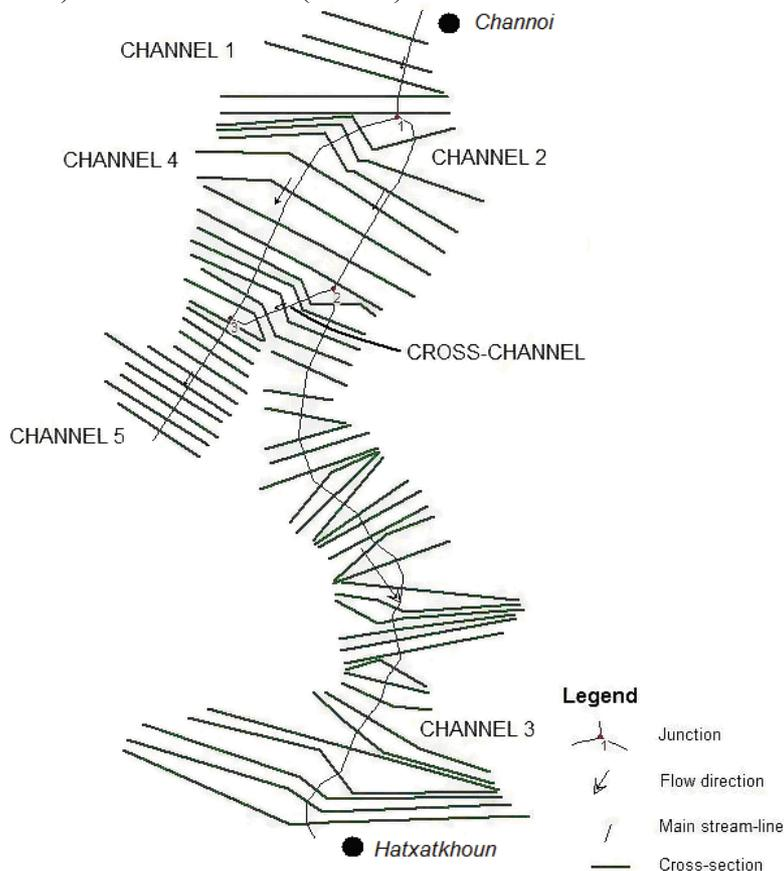
Figure 2. Cross-section alignment developed for both low and flooding discharge scenarios
