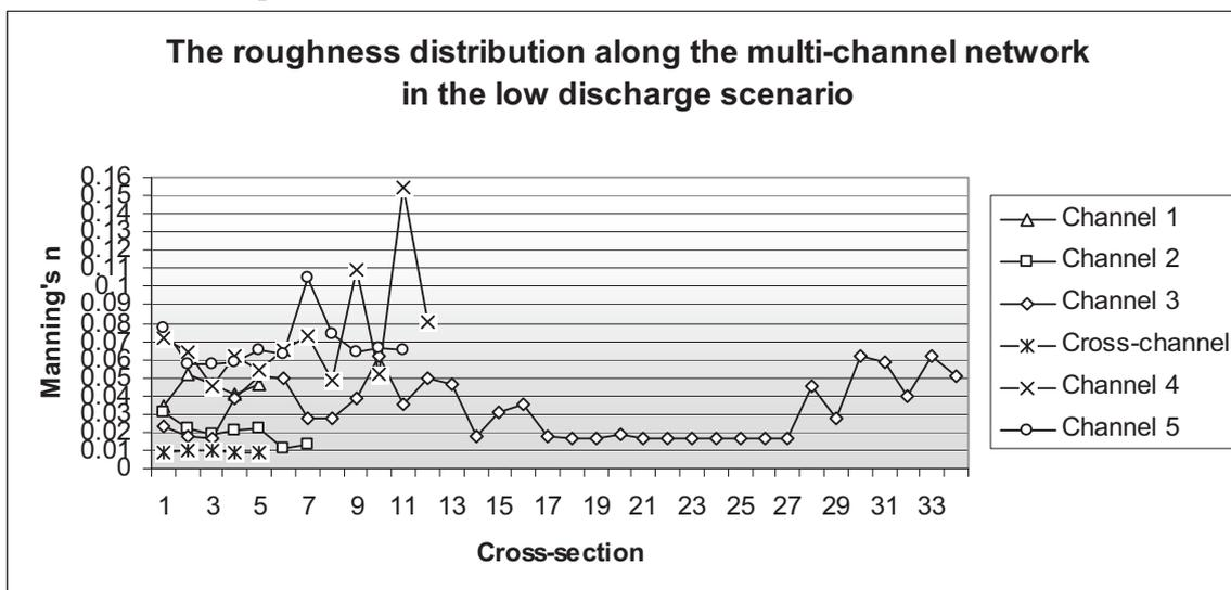
Figure 7. The hydraulic roughness distribution along the multi-channel network in the low discharge scenario
