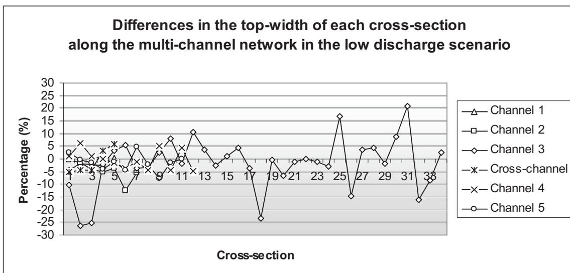
Figure 8. Comparison between the top-width derived from the HEC-RAS result versus SPOT image in the low discharge scenario
