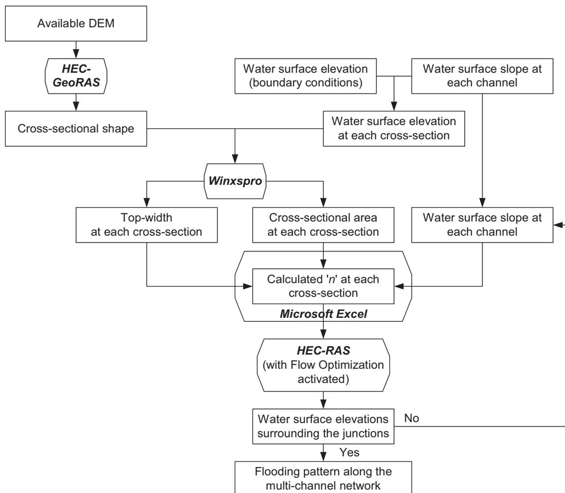
Figure 4. Routine to calibrate the HEC-RAS model for the flooding scenario
